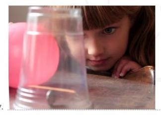
...and bring the statically charged balloon closer to the cup. The toothpick should move! The positively centred toothpick is attracted to the negatively charged balloon which makes the toothpick rotate and swing atop the coin!
